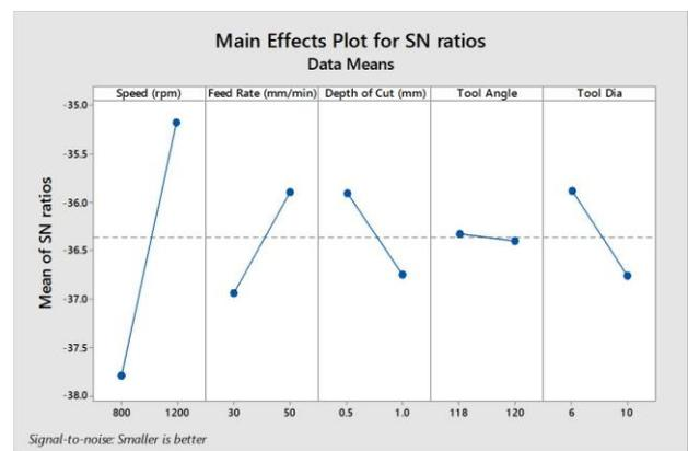
**Fig 1** Main effects plot of for S/N ratio values of Time taken
