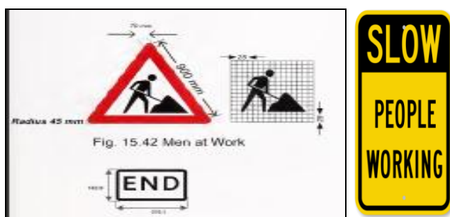
Fig 5.4 Sign Boards at Traffic Control Zone
