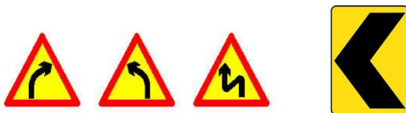
Fig 5.2 Curve sign boards and Chevron sign boards
