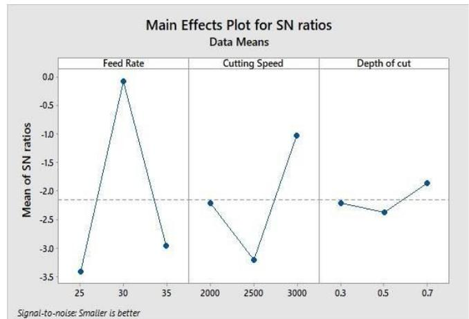
**Figure 1.** Effect of Feed, Speed & Depth of cut on Ra[2]
