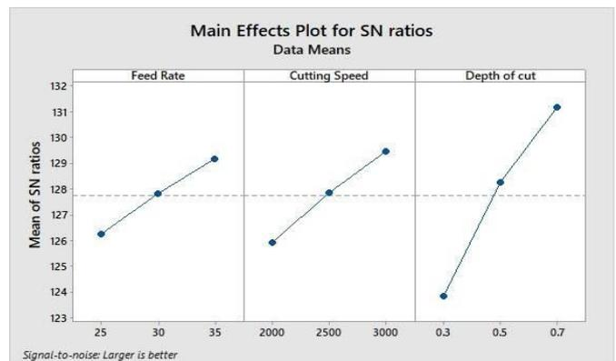
**Figure 2.** Effect of Feed, Speed & Depth of cut on MRR[2]
