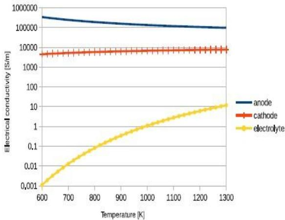
Figure 5: Electrical conductivity for SOFC anode, cathode and electrolyte although the decrease is substantial, electrolyte thickness is significantly smaller than one of the electrodes.
