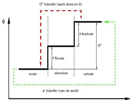
Figure 4: Charge transfer in electrode-electrolyte assembly of a SOFC.
