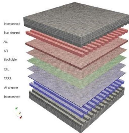
Figure 3: Regional and zonal decomposition of a mesh. It can be seen that regions (child meshes) from Figure are further divided into zones of uniform physical properties.
