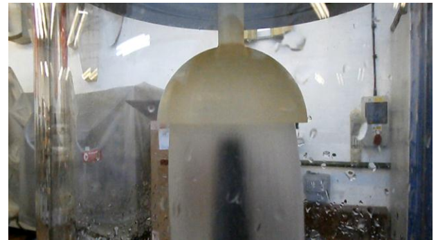
Figure 10: Exit Flow Direction for Hemispherical Vane
