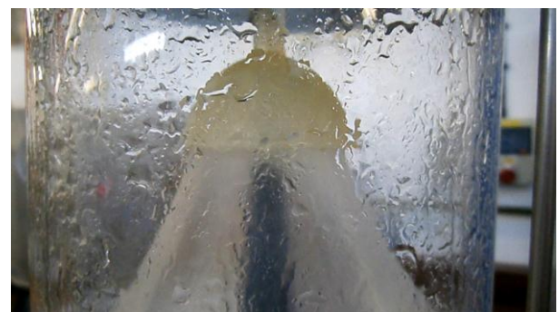
Figure 12: Exit Flow Direction for Egg Shaped Vane
