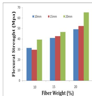
Graph 5: Effect of NaOH treated fiber length and weight percentage of flexural properties of sisal/bamboo composites
