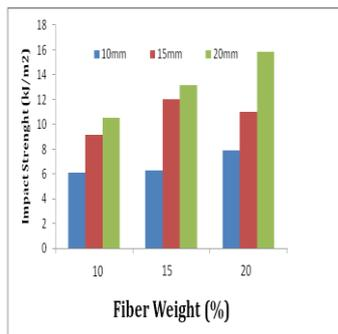
Graph 3: Effect of fiber length and weight percentage on impact properties of sisal/bamboo composites
