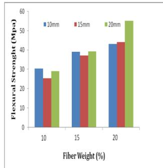
Graph 2: Effect of fiber length and weight percentage of flexural properties of sisal/bamboo composites
