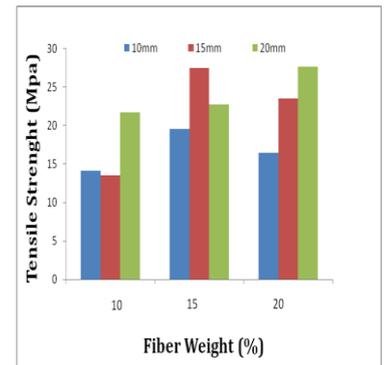
Graph 4: Effect of NaOH treated fiber length and weight percentage of tensile properties of sisal/ bamboo composites
