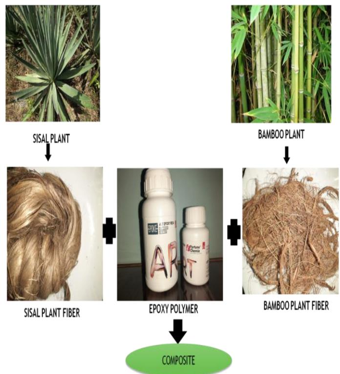
**Figure 1:** Represents the procedure of making Sisal and Bamboo Epoxy Composite
