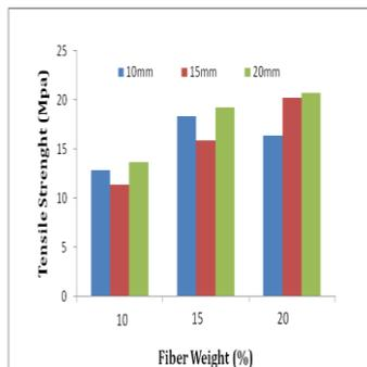
Graph 1: Effect of fiber length and weight percentage of tensile properties of sisal/ bamboo composites
