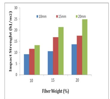
Graph 3: Effect of NaOH treated fiber length and weight percentage on impact properties of sisal/bamboo composites
