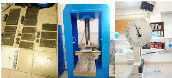
Fig (2) a. Samples after curing, b. Compression and bending machine, c. Impact machine
