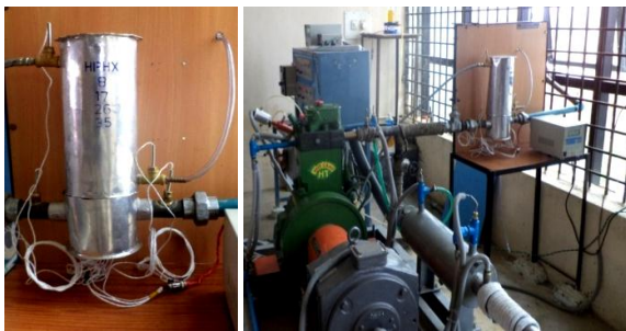
Figure 6: The instrumented and interfaced HPHX assembly
