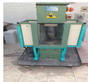
Fig. 2 Shape of the forge-forming machine after the installation of isolation box.
