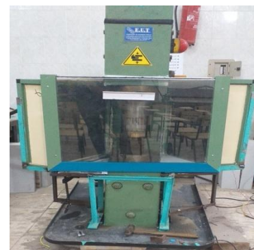
Fig 3. Shape of forge-forming machine after the installation of isolation box at angle of 120°.
