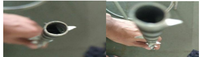
Fig -7: Pipe with Triangular Fin Insert.
