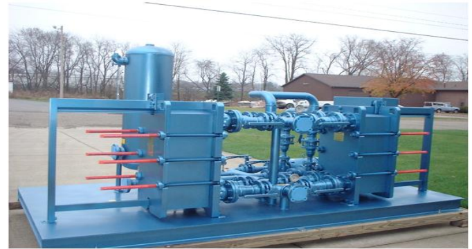
Fig 1.1 Liquid-to-Liquid Cooling Systems
