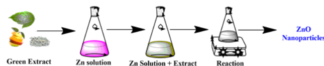
Figure 2: Schematic representation for the synthesis of ZnO nanoparticles
