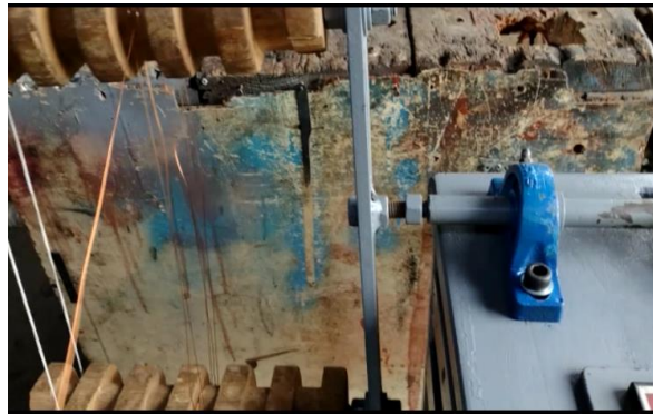
Figure 11: Placement of wire for winding
