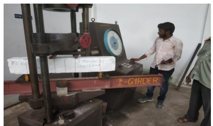
Figure 1: Testing of beam in UTM
