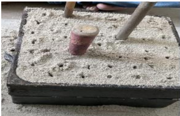
Fig -1: Mould preparation for the casting
