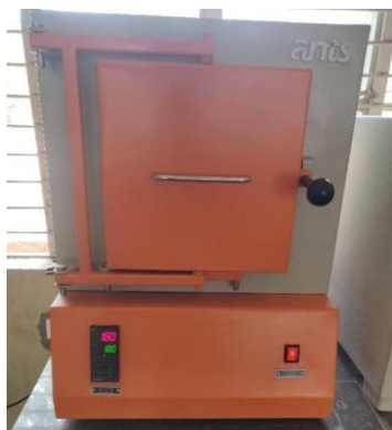
Fig -2: Muffle furnace used for heat treatment
