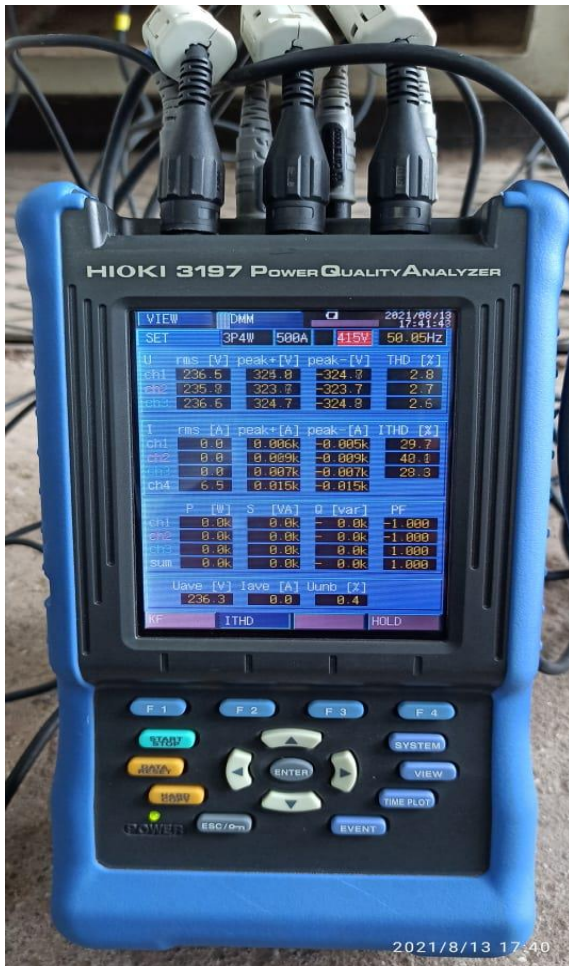
Fig. 3 Readings of Analyser when only School is "ON"
