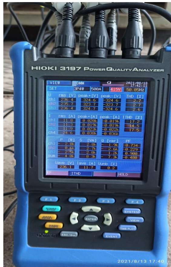
Fig. 4 Readings of Analyser when only Polytechnic is "ON"
