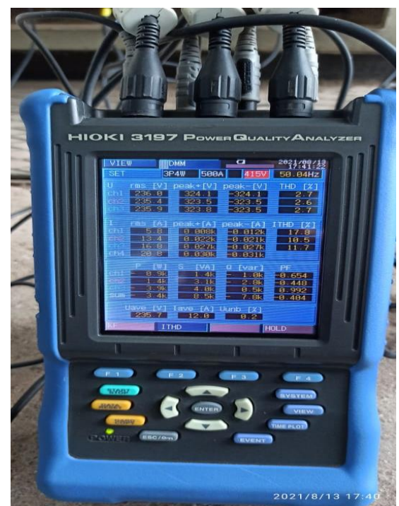
Fig. 5 Readings of Analyser when only Degree is "ON"
