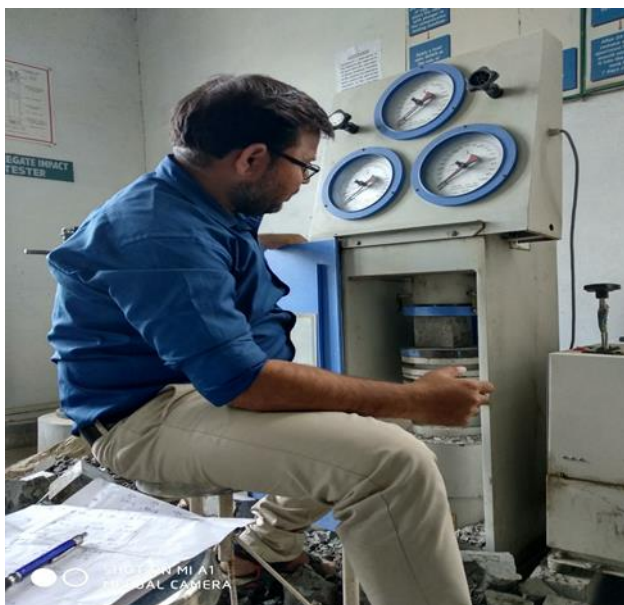
Fig -3: Compression Testing
