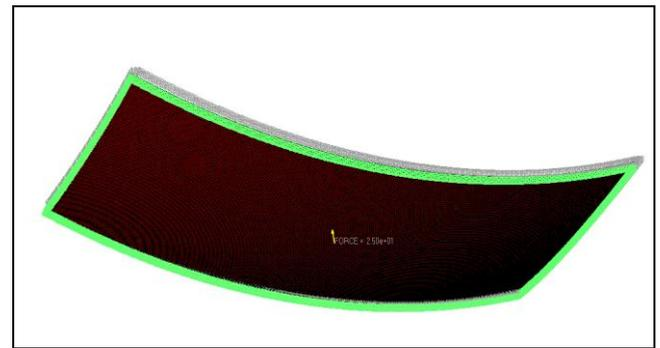
Fig-3: Load application and Boundary Condition
