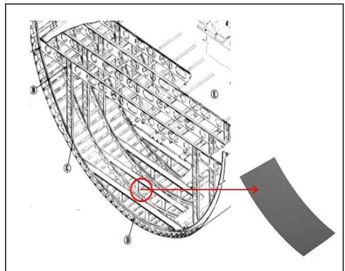
**Fig-1:** Fuselage Panel Considered For Analysis
