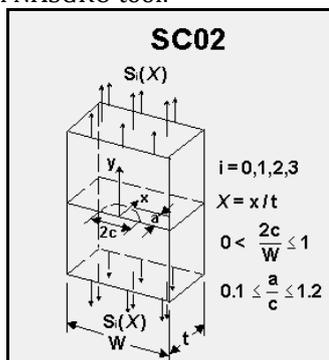
Fig-8: Crack growth model in NASGRO tool
