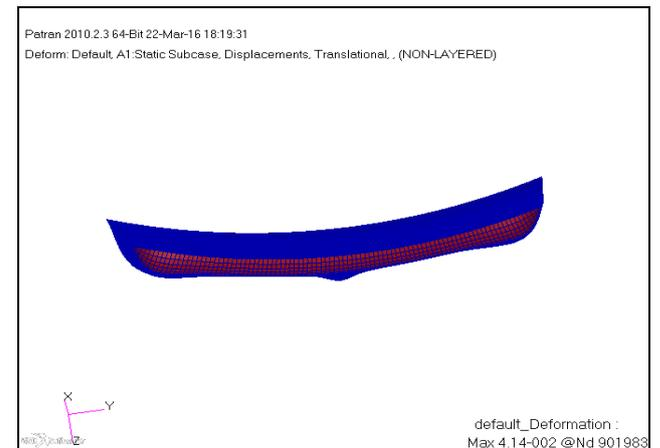
Fig-4: Panel Deformation due to applied load
