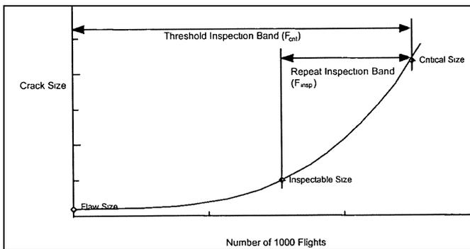
Fig-7: Crack growth curve
