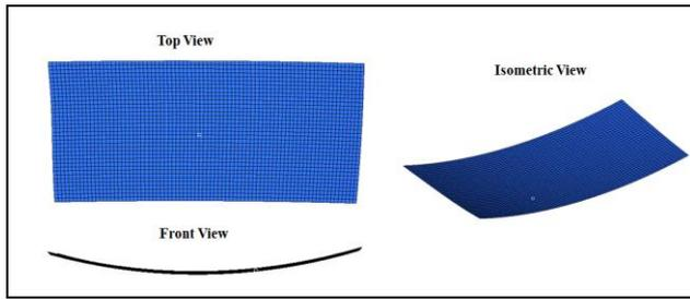
Fig-2: Aircraft Fuselage Panel Finite Element Model
