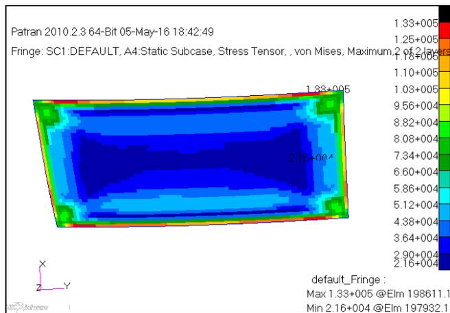
Fig-6: von Mises stress plot for debris impact
