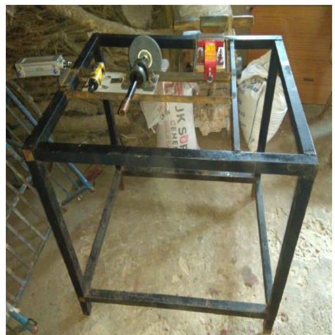
Fig 02:- Pneumatically powered grinding machine
