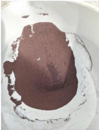
Figure-2: Copper coated MWCNT's brown
