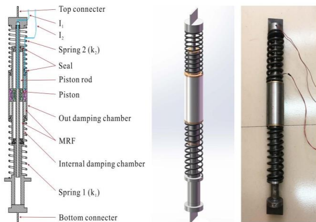
Fig-4: Variable stiffness MR damper proposed by author Huaxia Deng et al. [7].
