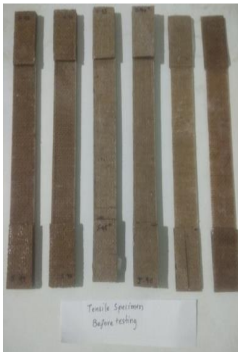
Fig -3: specimens prepared as per ASTM D3039
