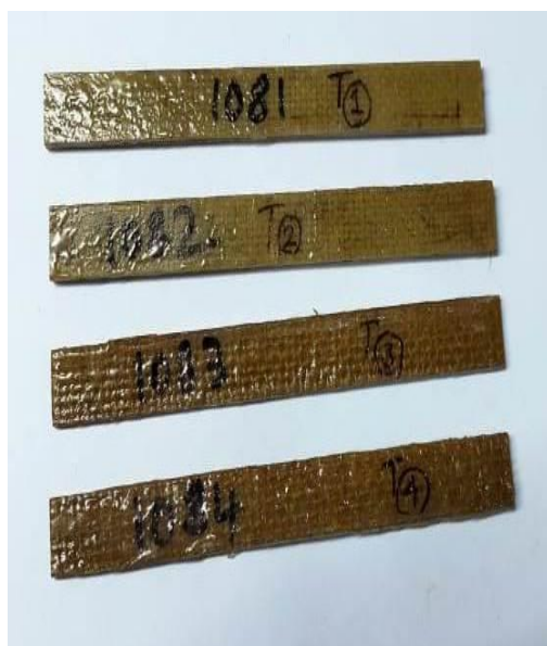
Fig -4: specimens prepared as per ASTM D790
