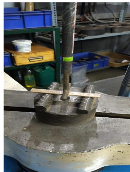
Fig -6: Flexural test arrangement at UTM
