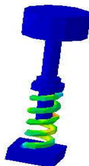
Fig: 6(b) Static Case Solution.1 - Von Miscellaneous stress (nodal values).2
