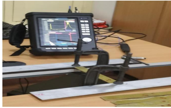
Fig no: 2 FRF vibration test setup.
