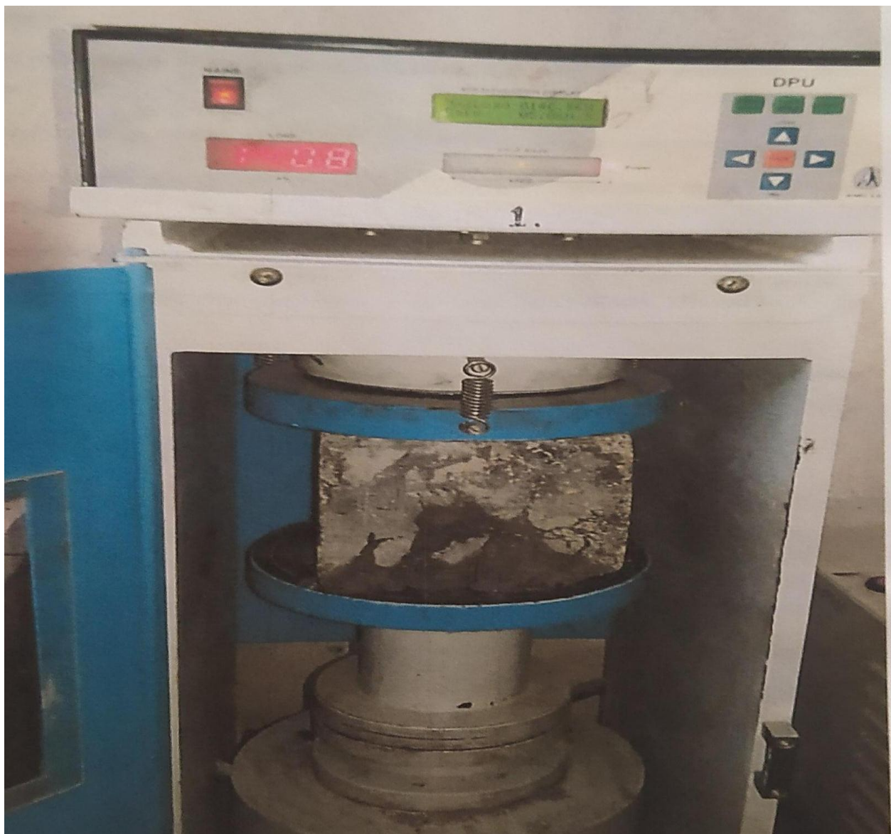
Fig: Compressive strength test on Coconut shell concrete
