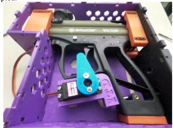
Figure -1: Paintball gun coupled into the box container
