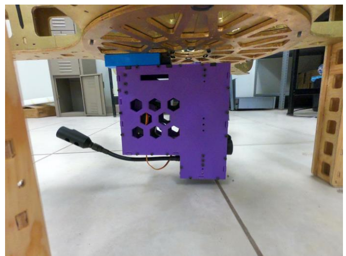
Figure 6: MESSD coupled under the hexacopter wooden frame.
