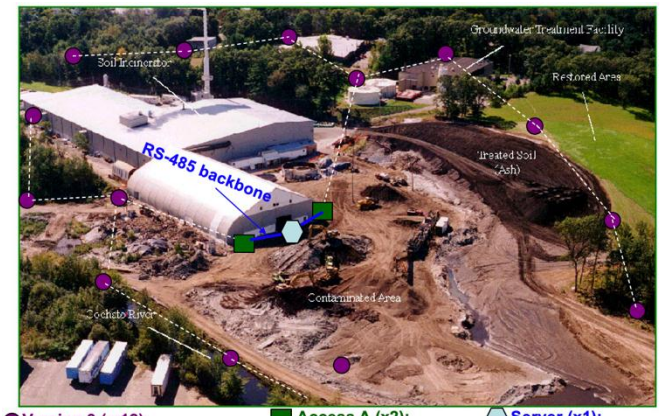
Fig. 30. Proposed deployment of integrated sensor system in an outdoor perimeter sensing and security location.
