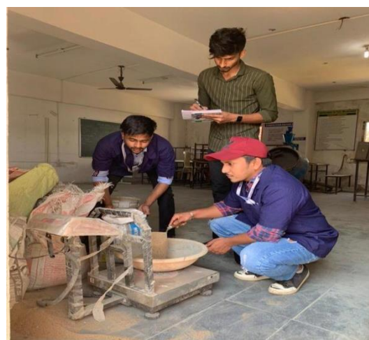
Fig-1 Batching of Aggregates
