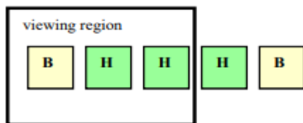
Fig -4: Hybrid markers: the center hybrid marker plays the role of Boundary markers for the left hybrid marker.
