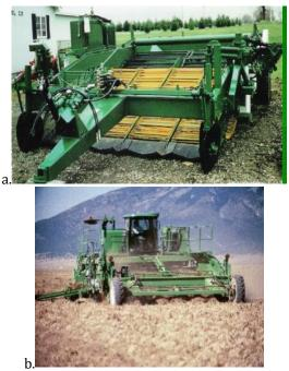
Figure 4.16. Windrower potato harvester (a) and Windrower harvester under operation (b)
