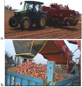
Figure 4.14. The tractor was drawn potato combine harvester (a) and potato combine loading system (b)
