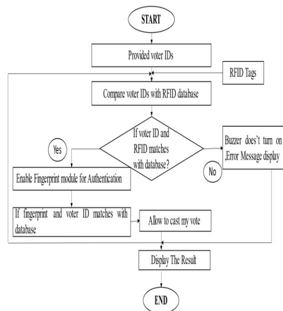
The flow chart explains the following process of the system which the connect to the circuit diagram. The RFID tag which stores the information of the voter. Then the RFID reader used to read the RFID tag.
