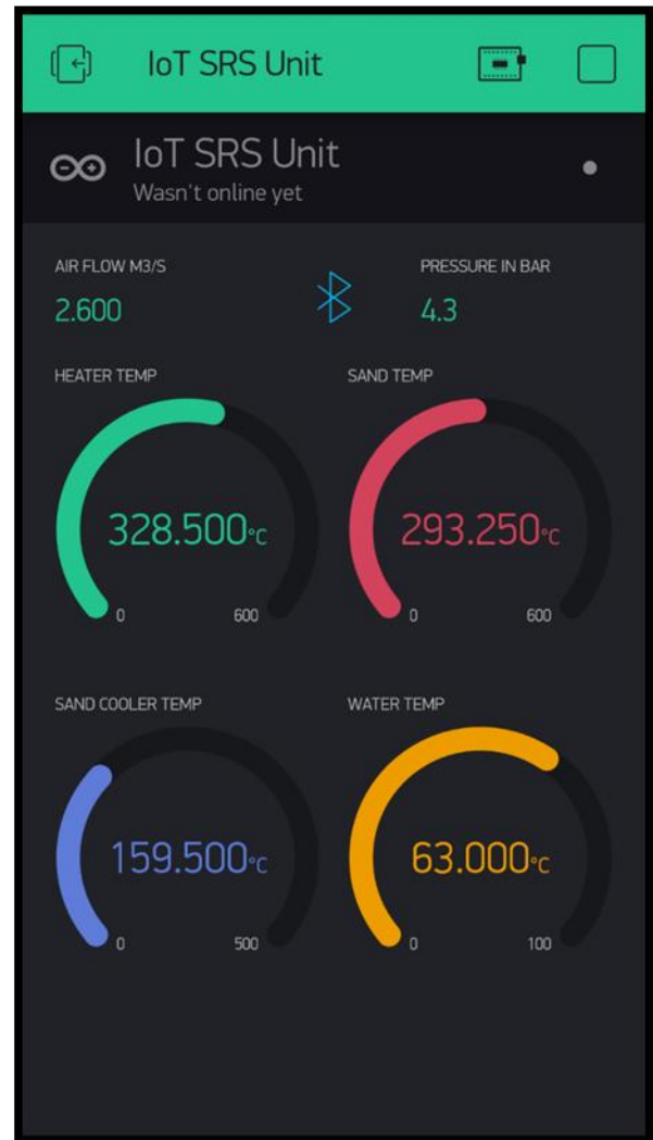
Fig -2: Online Monitoring of Smart Sand Reclamation System by use of BLYNK
