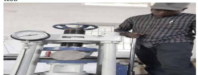
Figure 3: Uniaxial tensile test on concrete specimen
