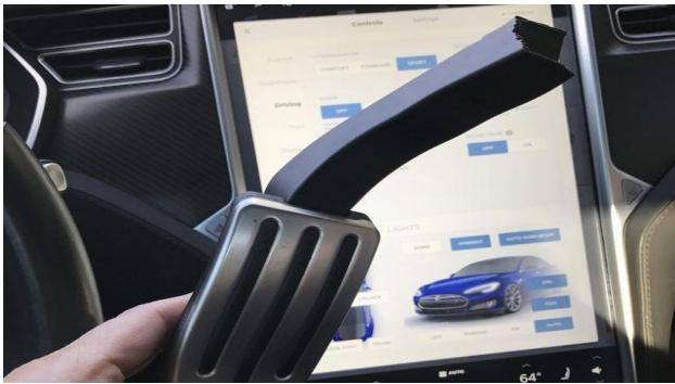
Fig-3: Failed Brake Pedal
