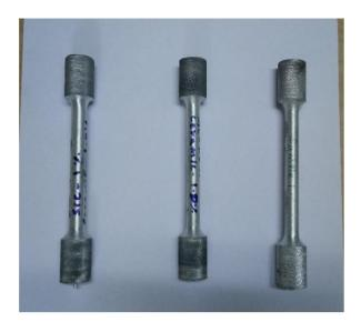
Fig-7: Tensile test specimen
