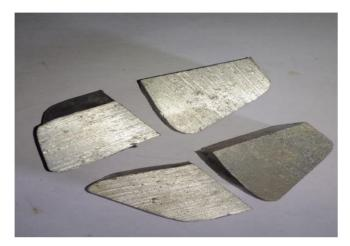
Fig-1 : Aluminium alloy LM25
