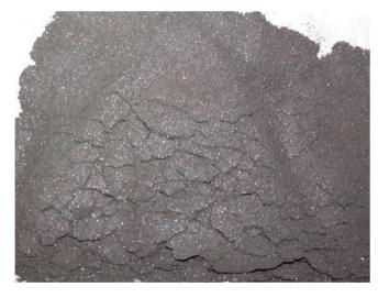
Fig-2 :Silicon carbide
