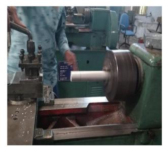
**Fig-6:** Machining of samples
