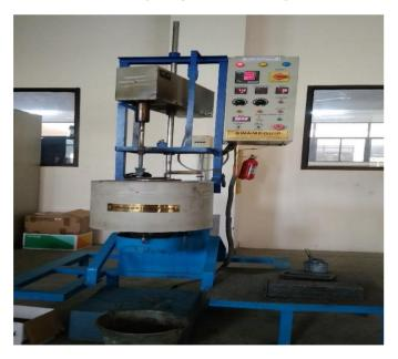
Fig- 4: Stir casting setup
