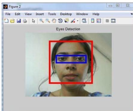
The system successfully detects the close eyes and alerts the driver to focus on driving by providing a beep.
