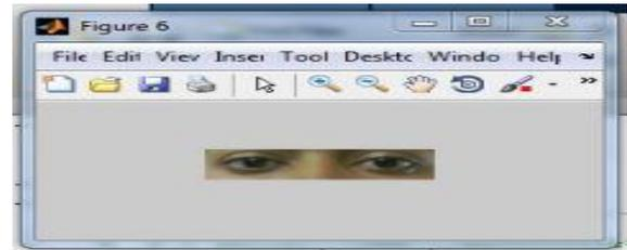
The system successfully detected the open eyes and didn't provide any alert sensing the drivers alertness since he was detected awake.
