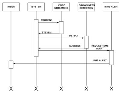
A Sequence diagram is in UNIFIED MODELLING LANGUAGE(UML). It is a kind of an interaction diagram that shows how process operate with one another and in what order. Sequence diagrams are sometimes called Event diagrams, Event scenarios and timing diagrams.
