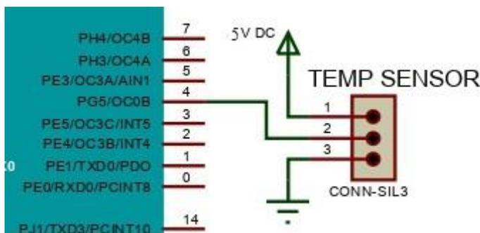
Fig -8: Connection of the temperature sensor with Arduino
