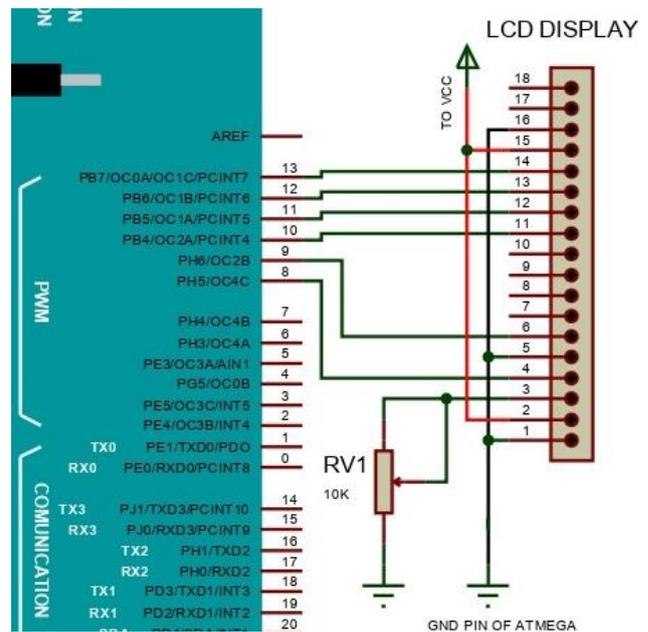
Fig -9: Connection of the LCD (16X2) with Arduino
