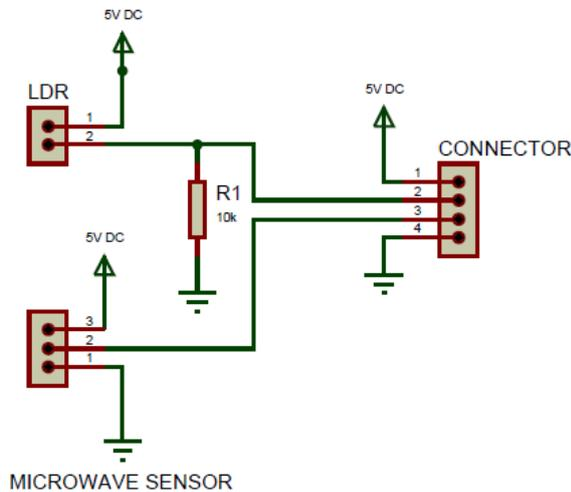
Fig -7: Internal connections of the Module
