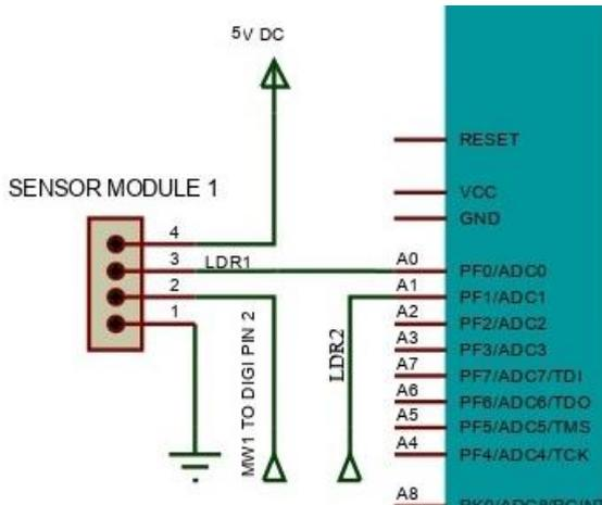
Fig -5: Connection of the module1 with Arduino
