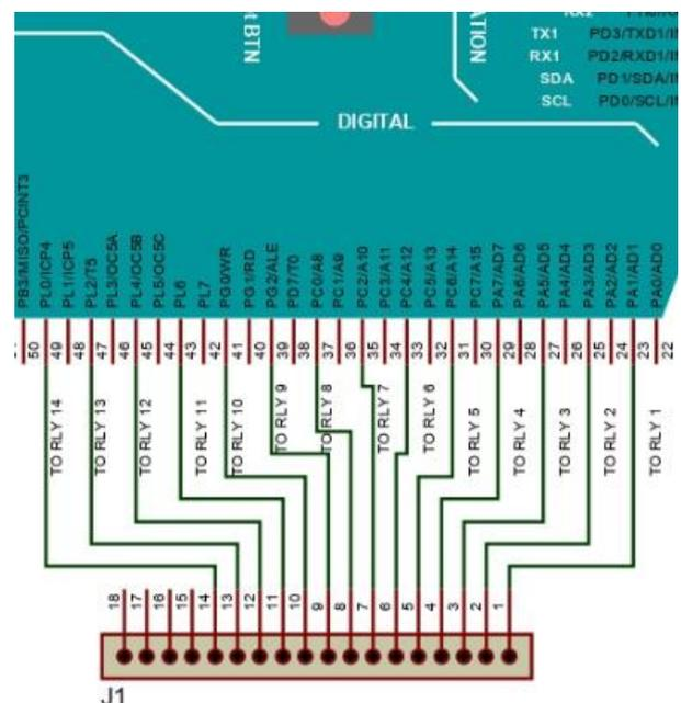
Fig -10: Connection of the Relays through Drivers with Arduino
