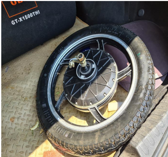
3.3.6 Fig No – 1 Wheel with a hub motor
