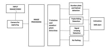
System Architecture of the Project is given above. It depicts that the flow of program will start by giving the system the input stream after which image processing will be done as a pre-processing step and then traffic rule violation detection is done. Once the violation is detected, the control goes to number plate recognition module and number plate is recognized by using OCR technique. In the End, the e-challan generated will be forwarded to the offender's contact.
