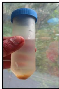
Fig -3: The CLEAs have settled at the bottom of the centrifuge tube
