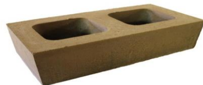
Fig.8. Brick made using excavation waste
