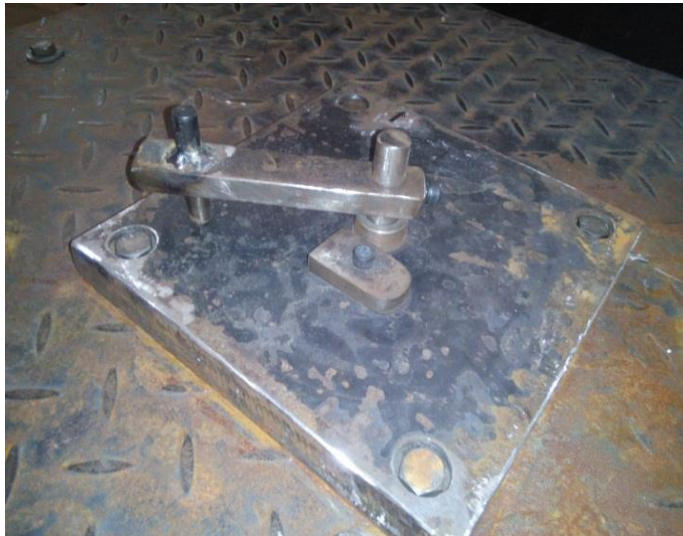
Fig.3- 2 New implemented design of die
