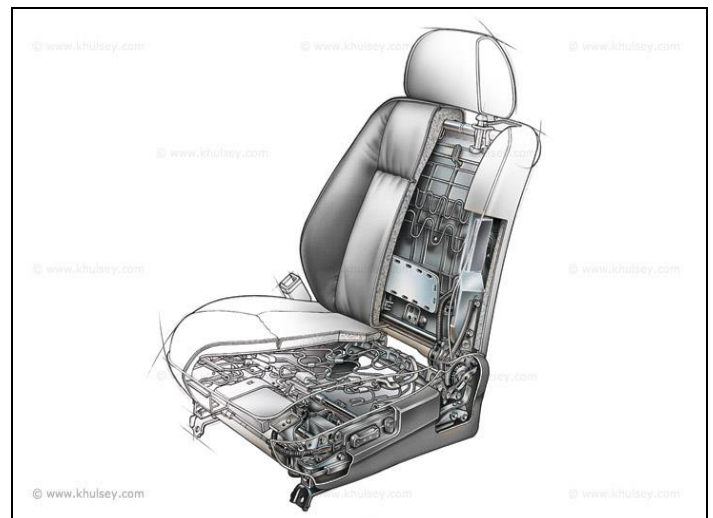
Fig.1. The zigzag spring use in car seat construction
