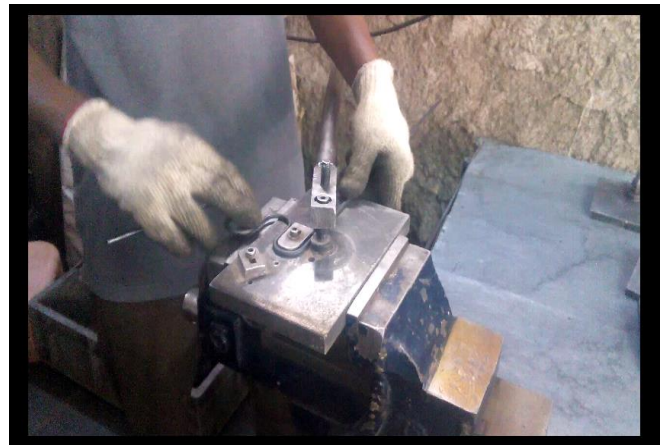
Fig.2- Existing method for zigzag spring manufacturing
