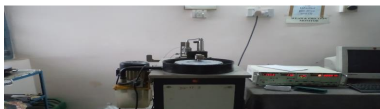
Fig.2.4 Wear testing using Pin-on-disc machine
