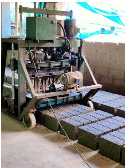
Fig-2: Moulding machine
