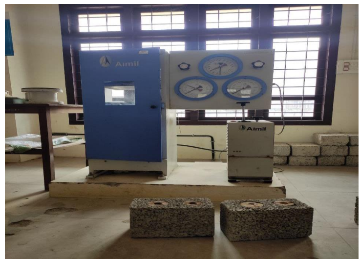
Fig 4 : Compression testing machine with Bamboo Bricks
