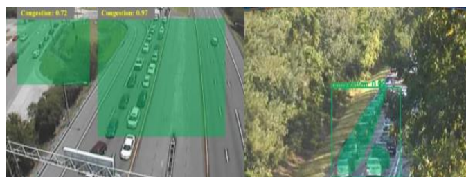
Fig -6: Traffic queue detection using YOLOv4(left) and Mask RCNN(right)[15]
