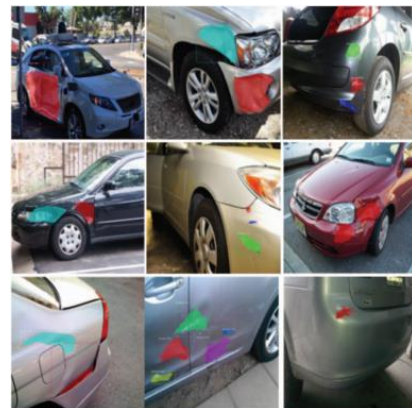
Fig -10: Detected damage on car body using Mask-RCNN[31]
