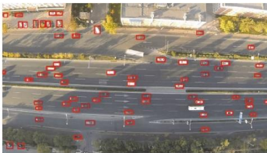
Fig -9: Vehicle localization using UAV images[30]
