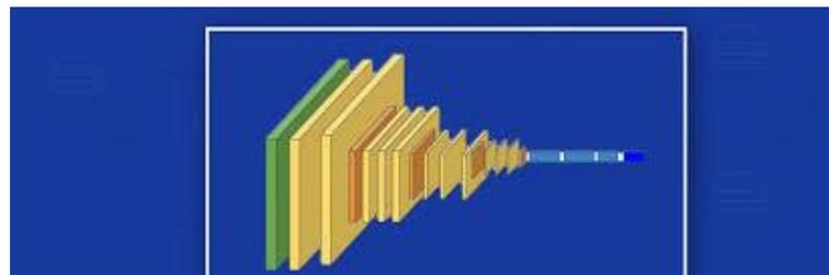
II Layer - A stride with 2 of size 2x2 is applied in pooling or sub-sampling layer resulting in reduction of image size to 14x14x6.
