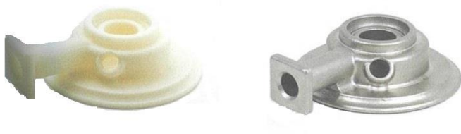
Fig-3: Application of FDM printing in investment casting patterns.
