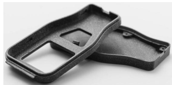
Fig-5: Application of FDM printing in Form & Fit Testing
