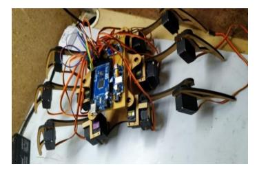
Microcontroller (Arduino mega) to servo connection was done by sending data parcels or data packets to servos and other sensors. Wireless communication through Bluetooth or WI-FI is used for communication between user and micro controller.
