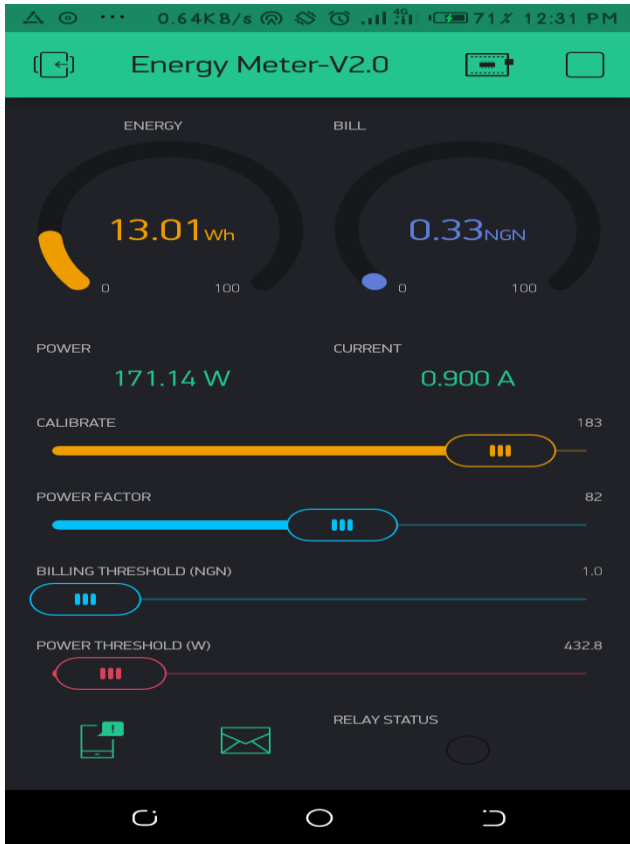
Figure 11: Display Readings at load
