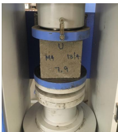
Fig -2: Compressive strength Test Apparatus
